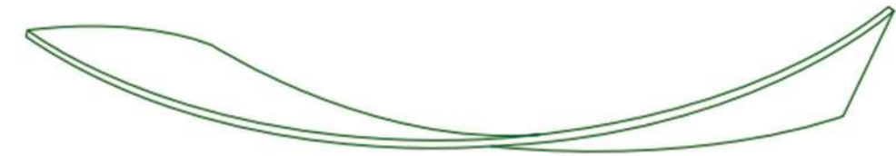
双S多曲弯钢化 Double S and multi-curved tempered
